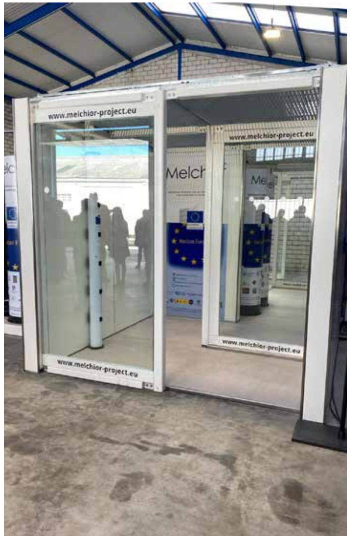
MELCHIOR blast-proof cabinet and detection technology.
